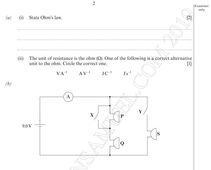
In the above circuit, buzzers P, Q and S are controlled using switches X and Y. The buzzers are identical and their resistances remain constant.
